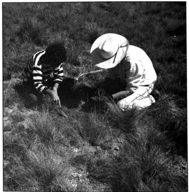
Photo 3. Conducting trowel test of soil
